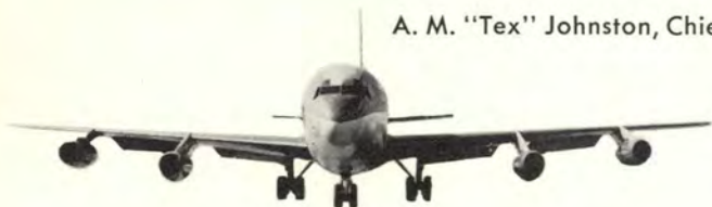
The 707 on final approach affords a good view of the four segment flap arrangement.
