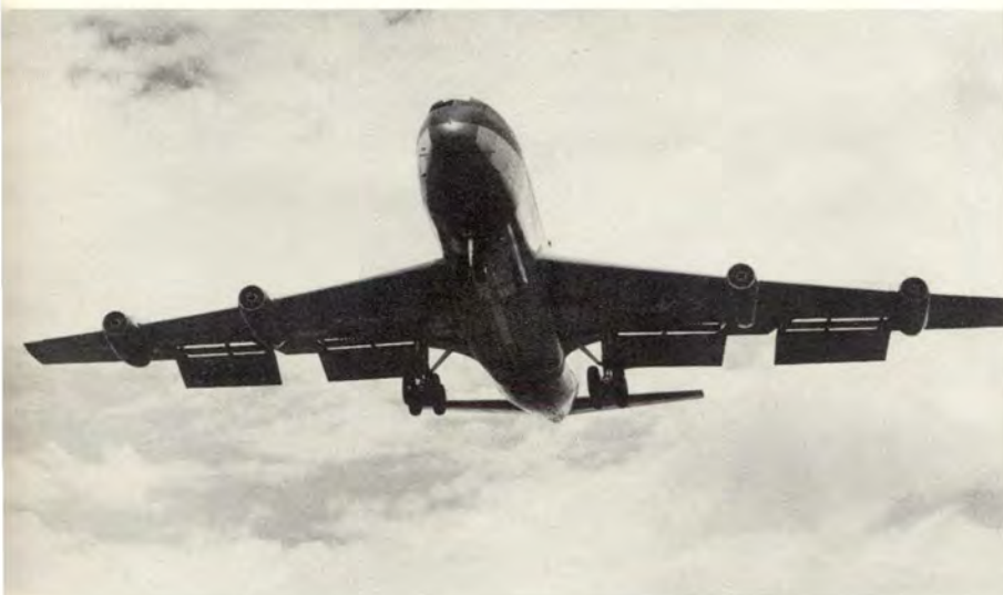
The 707 on final approach affords a good view of the four segment flap arrangement.
