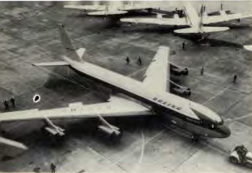
Above, the 707 in contrast to KC-97 tanker. Below, low slung engines are handy to work on.
