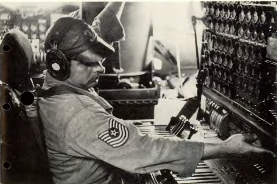
The engineer carries the ball on the engines, adjusting controls and monitoring instruments.
